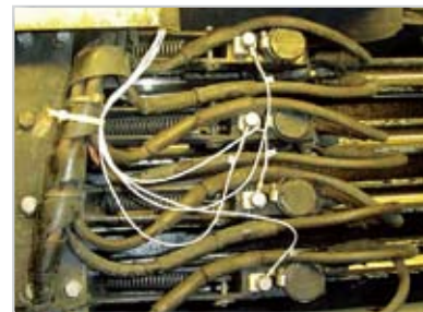
Collector arms with accelerometers attached
