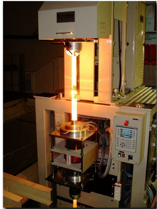
Draw tower top section : the glass perform is being heated in the induction furnace
