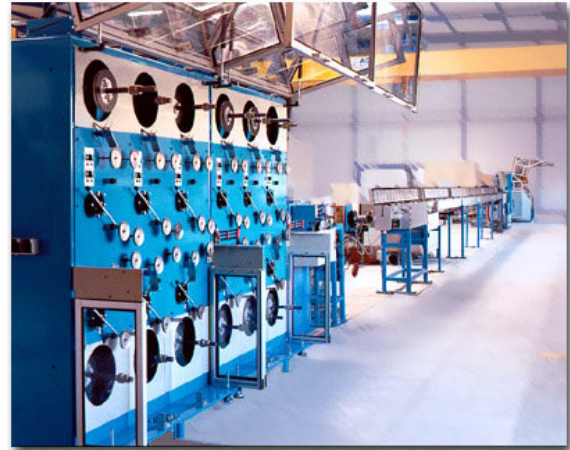
1000 m/min microtube secondary coating line
