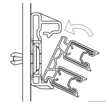
Faster, easier mounting due to a more rigid rail profile and uses 50% less rail hangers than comparable systems
