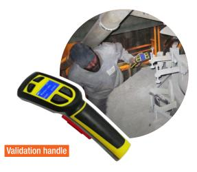
A 3-step trigger allows normal operation while half pressed. When released (fall, fear) or fully pressed (electric shock) all processes stop immediately.
